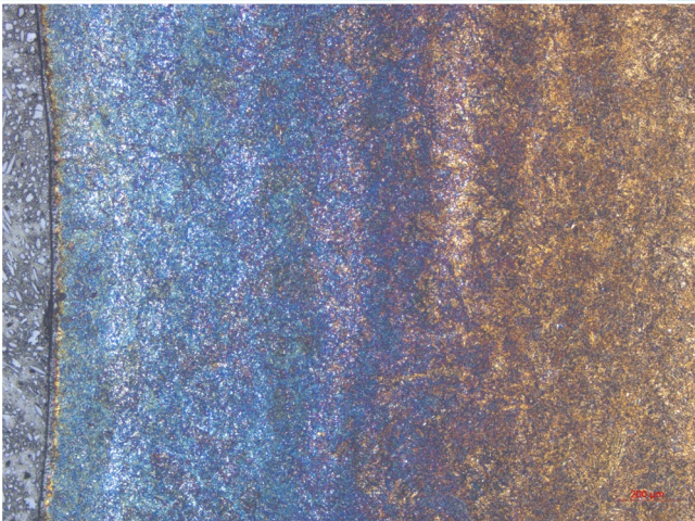
Etched with Nital 3%, BF, 50x
