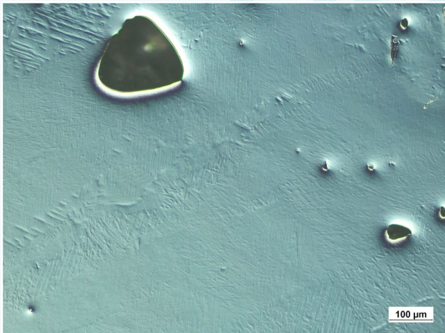
Ti6Al4V, Additive Manufacturing, DIC, 100x
