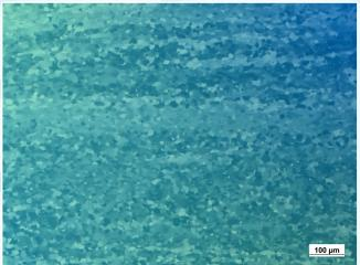
Pure Titanium, Grade 2, POL + Lambda Compensator, 100x
