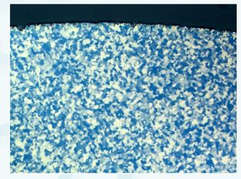
Pure Titanium, Grade 4, POL + Lambda Compensator, 200x
