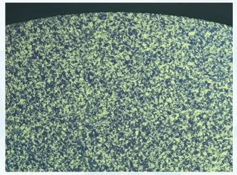
Pure Titanium, Grade 4, POL + Lambda Compensator, 100x
