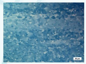
Pure Titanium, Grade 2, POL + Lambda Compensator, 200x
