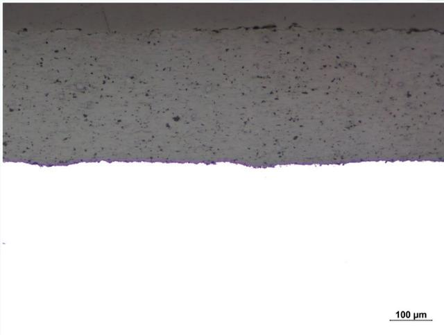
Al<sub>2</sub>O<sub>3</sub> coating on a steel substrate, BF, 100x
