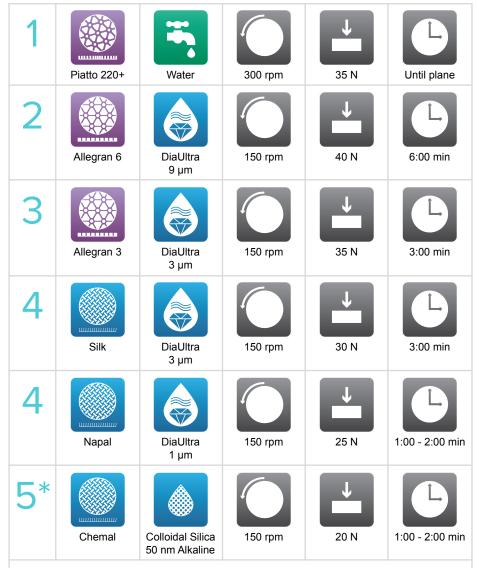
Times are stated for a 300 mm preparation system and 40 mm dia. samples. On a 250 mm system the times should be increased by 30%, on a 200 mm system by 100%.
