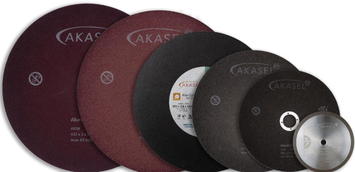
Aka-Cut 350 HV, Aka-Cut 500 HV and Aka-Cut 650 HV are fibre-reinforced wheels, well suited for cutting surface hardened workpieces with a hardness from 200-700 HV. The fibre-reinforcement strengthens the wheel and reduces breaking when subjected to pinching.
