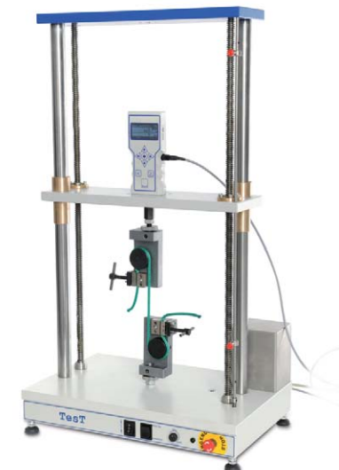
Motorized machine with force and displacement measurement
