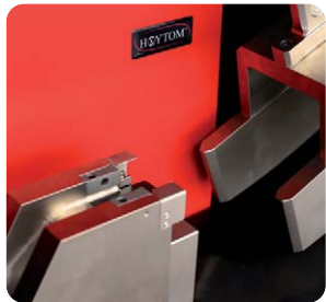
Charpy test tube holder
