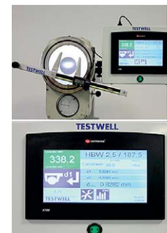
Retrofitting of hardness test machine
