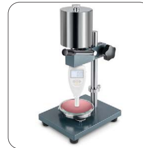
Shore hardness tester mounted on a measuring frame
