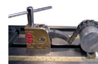
Kopal chain clamping system Ref. 50617
