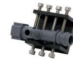
Chuck for irregular shape samples Ref. 51716
