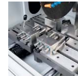
Motorized transversal table Ref. 50381
