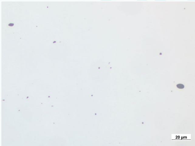
Low Alloy Steel 42CrMo4+QT, 330 HV, BF, 500x
